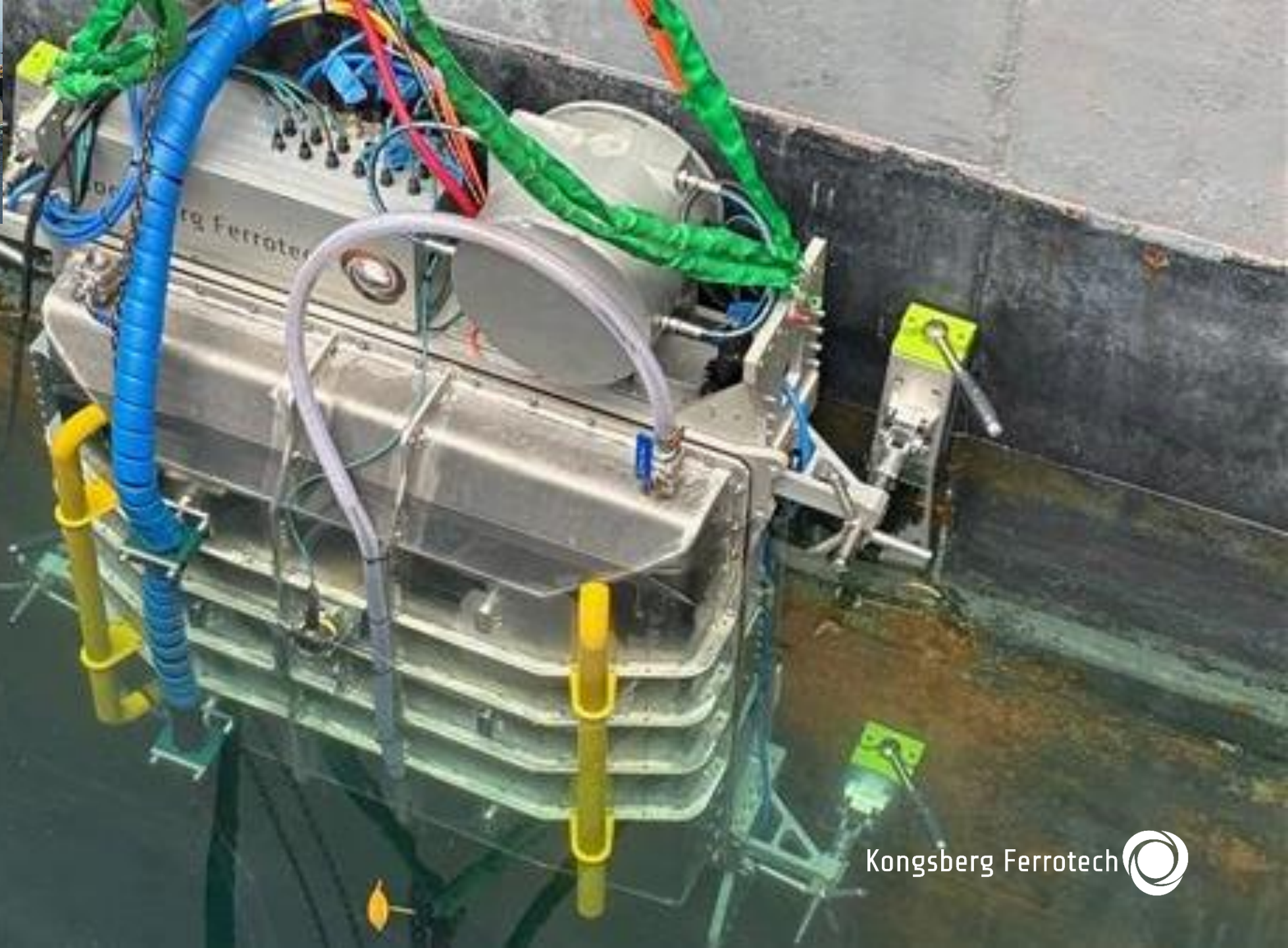
First fully robotic crack repair performed on a floating vessel Pearl Harbor, Hawaii, 2026 05 05
